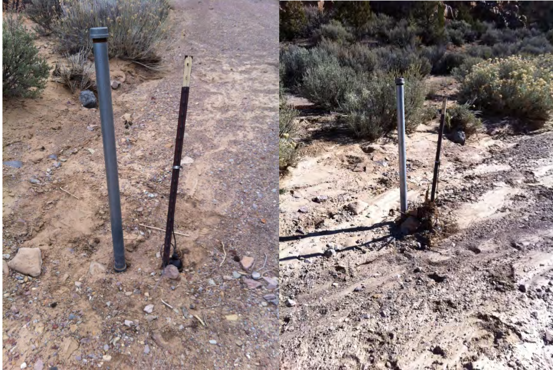
Photo of Crest Gauge and Single Stage Sampler initially set up and the same plugged by debris
